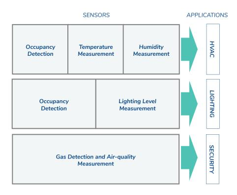
**Occupancy** sensors identify if a room is occupied or not while advanced occupancy sensors count the number of people in the area. Parameters that are used to measure their performance are their sensitivity and their resistance to "false triggering". Generally, there is a trade-off between the two which BEMs/HEMs developers need to manage.
